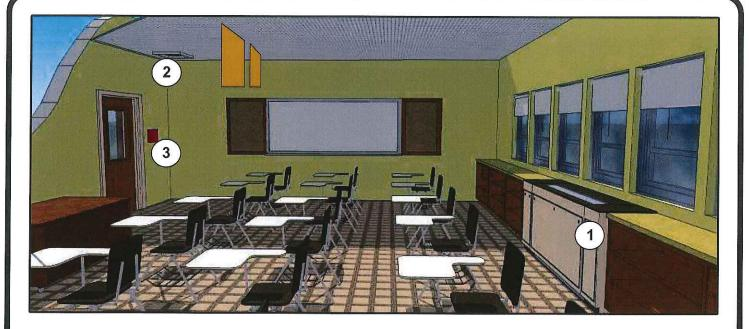
A unit ventilator 1 consists of a heating coil, fan assembly, dampers, filter and controls contained in a metal cabinet. Unit ventilators are usually located on the outside wall of classrooms, although they are sometimes suspended at or above the ceiling level.
