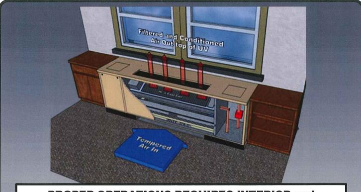
PROPER OPERATIONS REQUIRES INTERIOR and EXTERIOR AIR INTAKES and the TOP of the UNIT BE KEPT CLEAR WITH NO OBSTRUCTIONS AT ALL TIMES.
